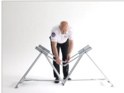
2) Release the telescopic shutter on the Upper Hinges (B) and fold down
