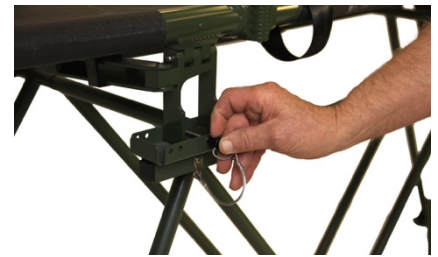
9) a: Push blue button to insert b: Push and pull to remove
