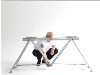
1) Remove the Quick Release Pin (F) on the Position Slider (G)
